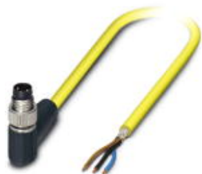
Sensor/Actuator cable, 3-position, PVC, yellow, shielded, Plug angled M8, on free cable end, Cable length: 2 m
