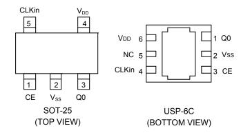
$^{\star}$  The dissipation pad (TAB) of the bottom view of the USP-6C package should be connected to the  $V_{\rm SS}$  (No. 2) pin.
