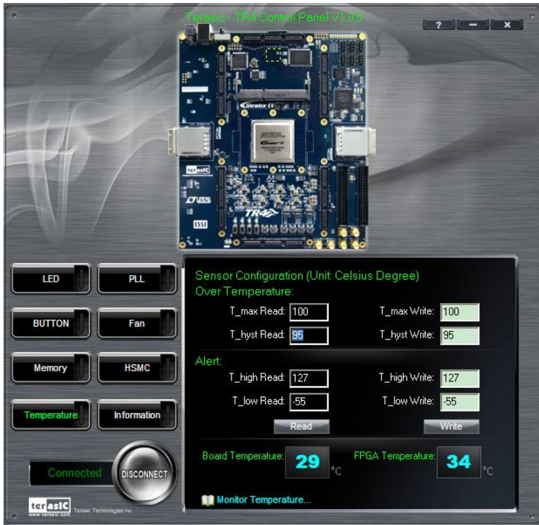
Figure 3-9 Accessing the Temperature Sensor through Control Panel
