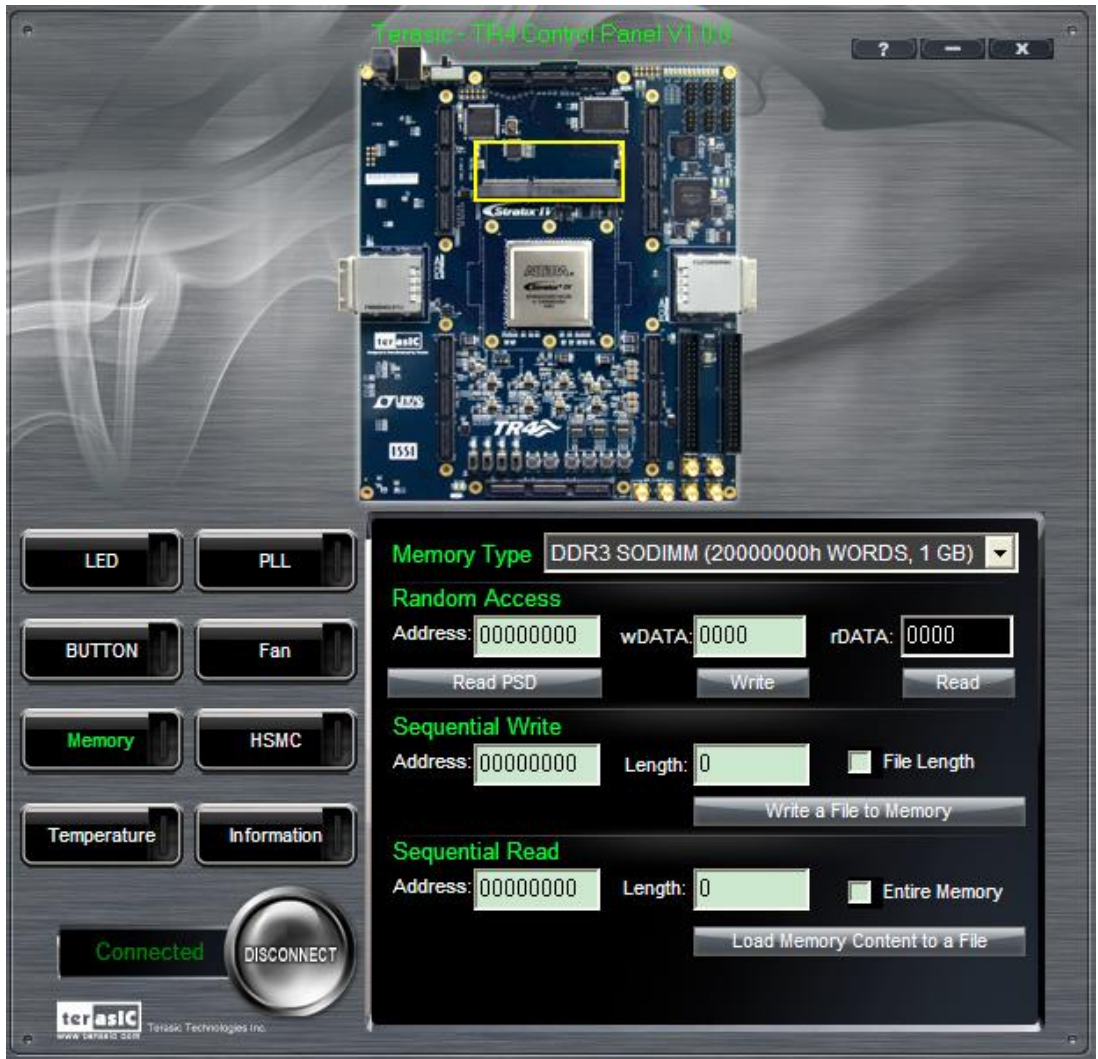
Figure 3-7 Access DDR3 SO-DIMM Memory
