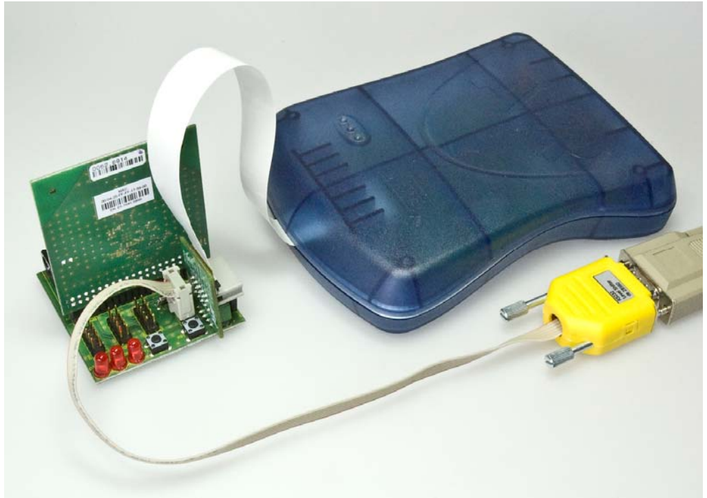
Figure 3-1. Atmel REB-CBB connected to an Atmel REB231ED with an RS232 cable plugged in and an Atmel AVR JTAGICE mkII programming interface.
