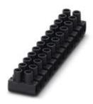
Polypropylene Europe terminal strip, black, for connecting solid conductors and stranded conductors with and without ferrules with a cross section of 0.5 to 4 mm<sup>2</sup>
