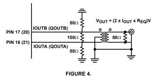
$V_{OUT}$  = 2 x  $I_{OUT}$  x  $R_{EQ}$ , where  $R_{EQ}$  is ~12.5 $\Omega$ .
