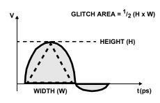
FIGURE 1. OUTPUT SETTLING TIME DIAGRAM
