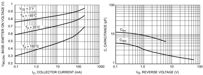
Figure 5. Base–Emitter Turn–ON Voltage vs. Collector Current
