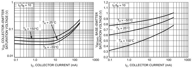
Figure 1. Collector–Emitter Saturation Voltage vs. Collector Current
