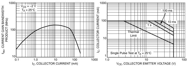
Figure 7. Current Gain Bandwidth Product vs. Collector Current
