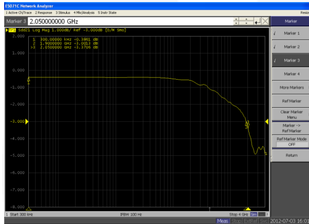
Figure 17. MHL Path SDD21 Insertion Loss Curve
