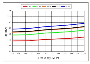
Figure 8. Idd vs Frequency
