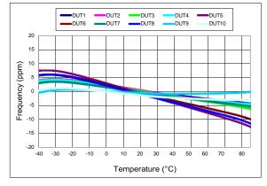
Figure 9. Frequency vs Temperature, 1.8V
