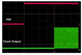
Figure 17. Startup Waveform vs. Vdd
