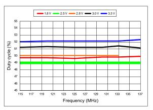
Figure 11. Duty Cycle vs Frequency
