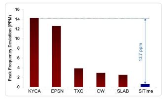
Figure 6. Shock Robustness<sup>[6]</sup>
