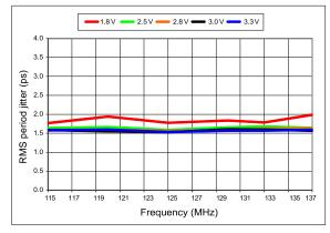
Figure 10. RMS Period Jitter vs Frequency
