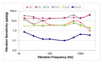
Figure 5. Vibration Robustness<sup>[5]</sup>
