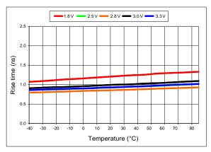
Figure 12. 20%-80% Rise Time vs Temperature
