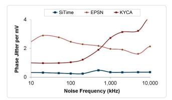
Figure 4. Power Supply Noise Rejection<sup>[4]</sup>
