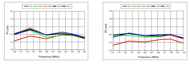
Figure 14. RMS Integrated Phase Jitter Random (12 kHz to 20 MHz) vs Frequency<sup>[9]</sup>
