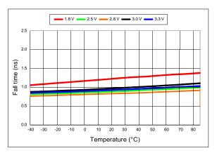
Figure 13. 20%-80% Fall Time vs Temperature
