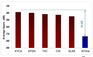
Figure 3. Electro Magnetic Susceptibility (EMS)<sup>[3]</sup>
