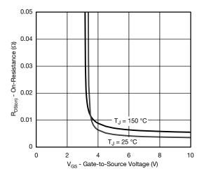
On-Resistance vs. Gate-to-Source Voltage
