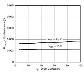
On-Resistance vs. Drain Current
