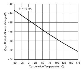
**Drain Source Breakdown vs. Junction Temperature**
