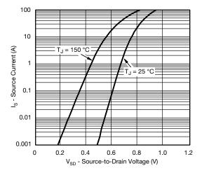
**Source Drain Diode Forward Voltage**
