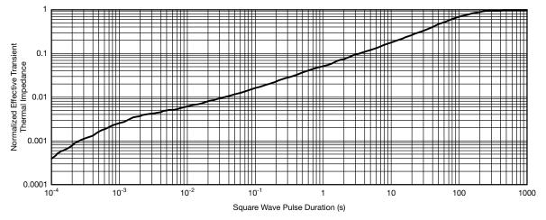
Normalized Thermal Transient Impedance, Junction-to-Ambient
