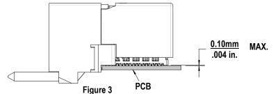
There should be no broken stand-offs along the perimeter of the part (an indication of over-pressing).
