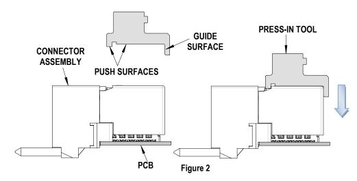
3. Using the application tool and an appropriate press, seat the Orthogonal Direct Ram module until there is less than 0.10mm (.004 in) clearance between the bottom of the plastic housing and the surface of the PCB. See Figure 3.
