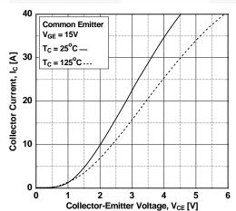
Figure 5. Saturation Voltage vs. Case
