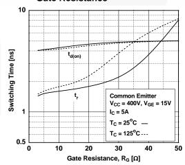
Figure 13. Turn-off Characteristics vs.
