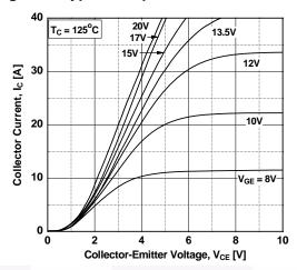
**Figure 4. Transfer Characteristics**
