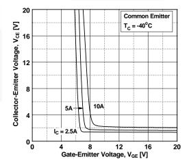
Figure 7. Saturation Voltage vs. V<sub>GE</sub>
