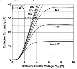
Figure 3. Typical Saturation Voltage Characteristics
