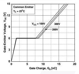
Figure 12. Turn-on Characteristics vs.
