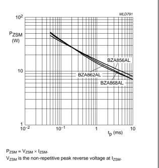
Fig.3 Maximum non-repetitive peak reverse power dissipation as a function of pulse duration (square pulse).
