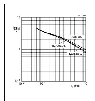
Fig.2 Maximum non-repetitive peak reverse current as a function of pulse time.
