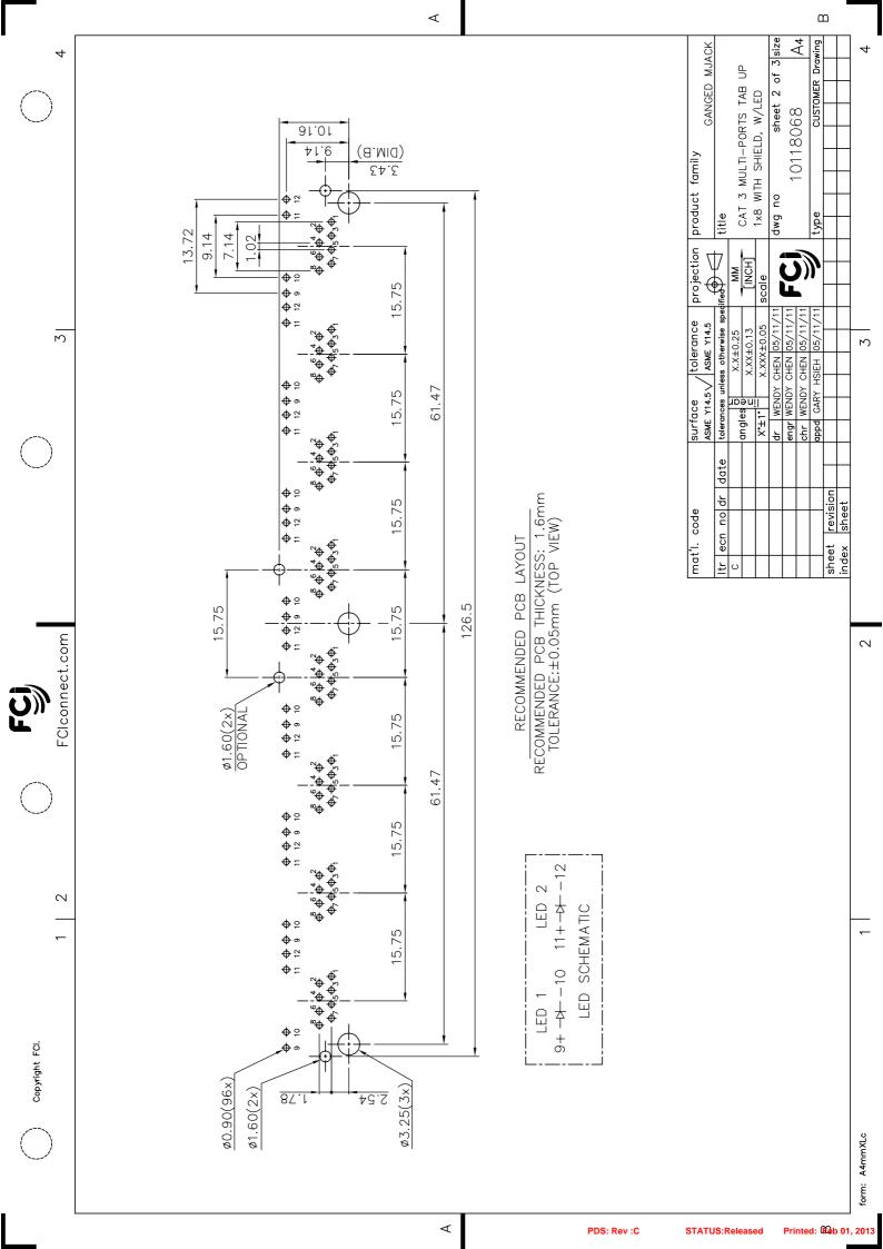
$_{\Omega}$ Ą sheet 3 of 3 size CUSTOMER Drawing GANGED MJACK CAT 3 MULTI-PORTS TAB UP 0 : WITHOUT PANEL GROUND 3 : TOP/RIGHT/LEFT 3 SIDES WITH PANEL GROUND 1x8 WITH SHIELD, W/LED 10118068 product family OPTIONAL RIGHT / LEFT SHIELD TAB 0 : WITHOUT LED
