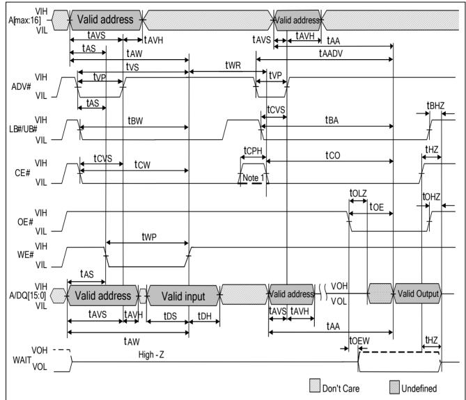
Notes: 1.When configured for synchronous mode (BCR[15] = 0), CE# must remain HIGH for at least 5ns (tCPH) to schedule the appropriate refresh interval. Otherwise, tCPH is only required after CE#-controlled WRITEs.
