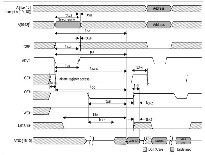
Note : A [19:18] = 00b to read RCR, 10b to read BCR , and 01b to read DIDR.
