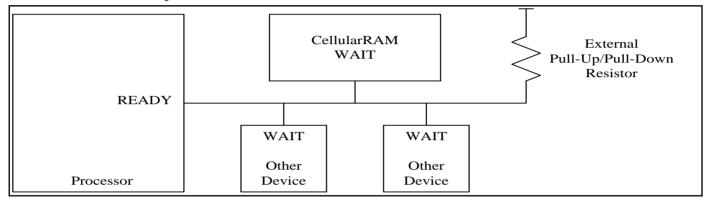
When a burst READ or WRITE operation has been initiated, WAIT goes active to indicate that the ADMUX PSRAM device requires additional time before data can be transferred. For READ operations, WAIT will remain active until valid data is output from the device. For WRITE operations, WAIT will indicate to the memory controller when data will be accepted into the ADMUX PSRAM device. When WAIT transitions to an inactive state, the data burst will progress on successive clock edges.
