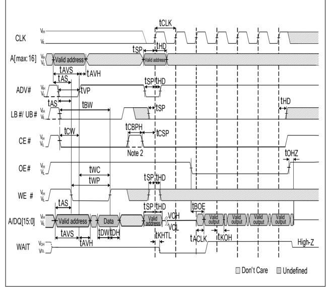
Notes: 1.Non-default BCR settings for asynchronous WRITE, with ADV# LOW, followed by burst READ: fixed or variable latency, latency code 2 (3 clocks), WAIT active LOW, WAIT asserted during delay.
