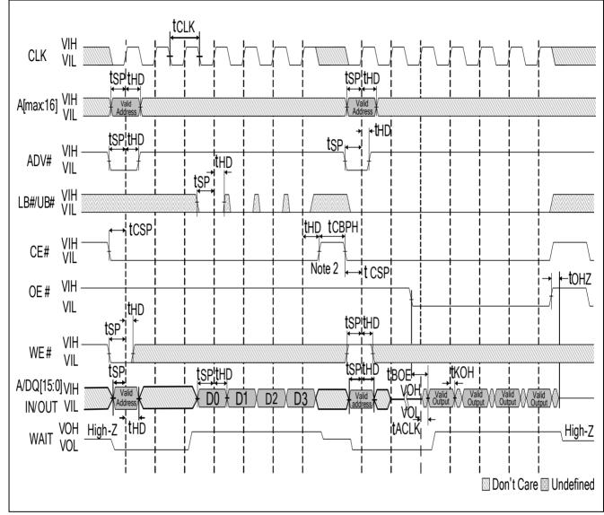
Notes: 1.Non-default BCR settings for burst WRITE followed by burst READ: fixed or variable latency, latency code 2 (3 clocks), WAIT active LOW, WAIT asserted during delay.
