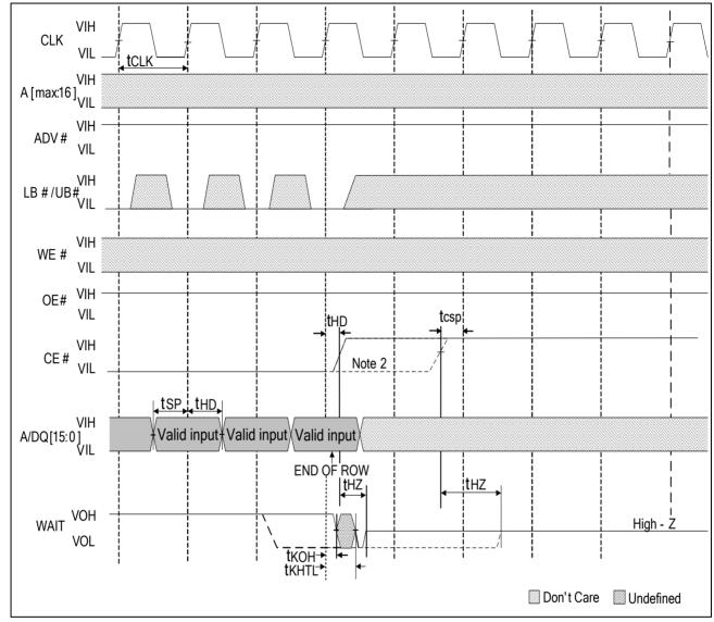
Notes: 1.Non-default BCR settings for burst WRITE at end of row: fixed or variable latency, WAIT active LOW, WAIT asserted during delay (shown as solid line).
