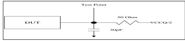
Notes: All tests are performed with the outputs configured for default setting of half drive strength (BCR[5:4] = 01b).
