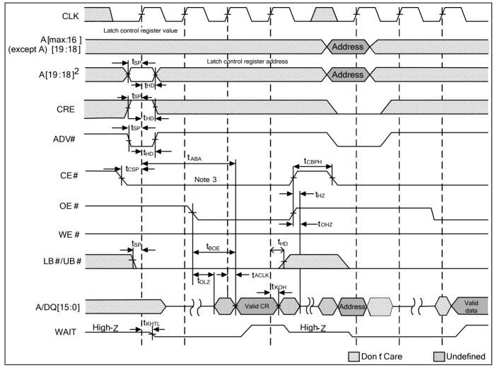
Notes :1.Non-default BCR settings for synchronous mode register READ followed by READ ARRAY operation : Latency code2(3 clocks) : WAIT active LOW;WAIT asserted during delay.
