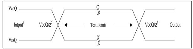
Notes:1.AC test inputs are driven at VccQ for a logic 1 and VssQ for a logic 0. Input rise and fall times (10% to 90%) <1.6ns. 2.Input timing begins at VccQ/2.
