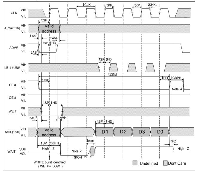
Notes: 1.Non-default BCR settings for burst WRITE operation in fixed latency mode: fixed latency, latency code 2 (3 clocks), WAIT active LOW, WAIT asserted during delay, burst length 4, burst wrap enabled.
