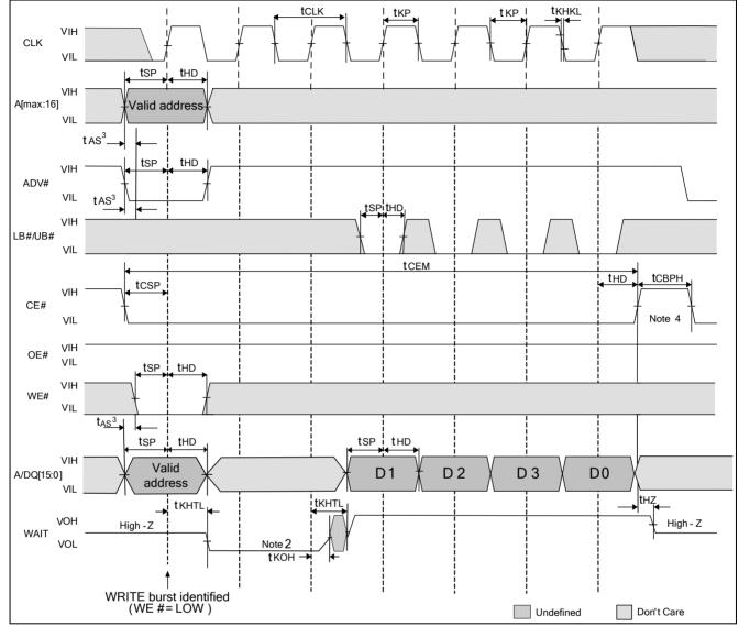
Notes: 1.Non-default BCR settings for burst WRITE operation in variable latency mode: latency code 2 (3 clocks), WAIT active LOW, WAIT asserted during delay, burst length 4, burst wrap enabled.
