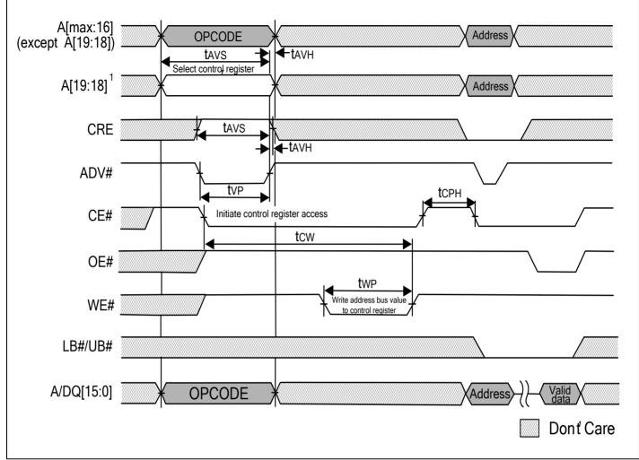
Notes: 1. A[19:18] = 00b to load RCR, and 10b to load BCR.
