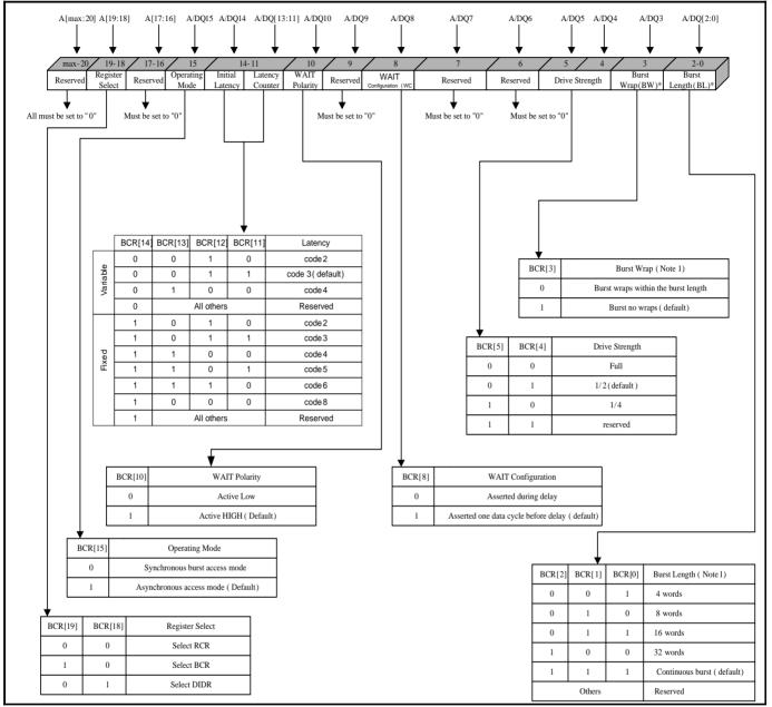
Notes: 1. Burst wrap and length apply to both READ and WRITE operations.
