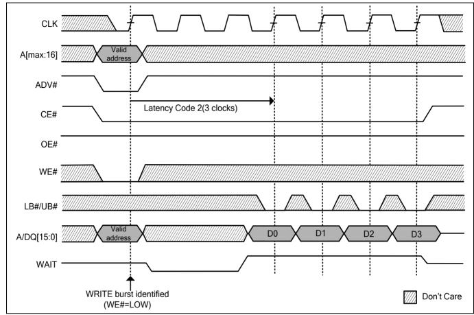
Note : Non-default BCR settings for burst mode WRITE (4-word burst) : fixed or variable latency , latency code 2(3 clocks) , WAIT active LOW, WAIT asserted during delay.
