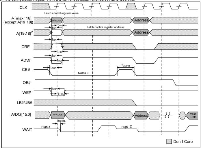
Notes: 1.Non-default BCR settings for synchronous mode configuration register WRITE followed by READ ARRAY operation: latency code 2 (3 clocks), WAIT active LOW, WAIT asserted during delay.
