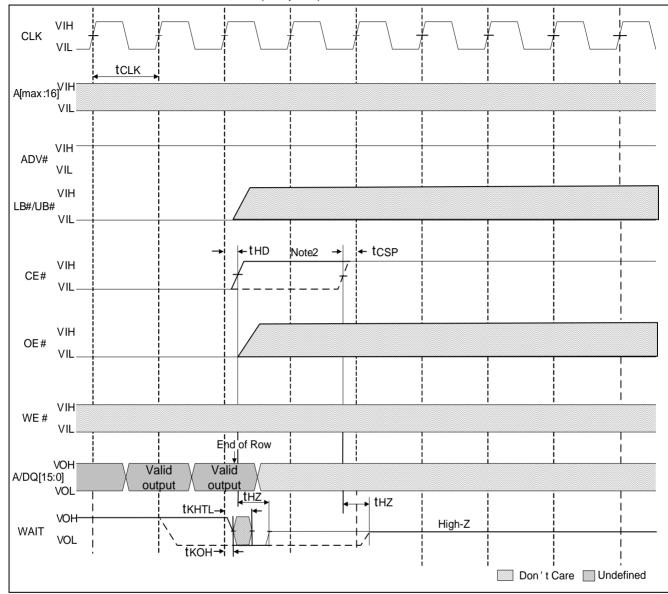
Notes: 1.Non-default BCR settings for burst READ at end of row: fixed or variable latency, WAIT active LOW, WAIT asserted during delay (shown as solid line).
