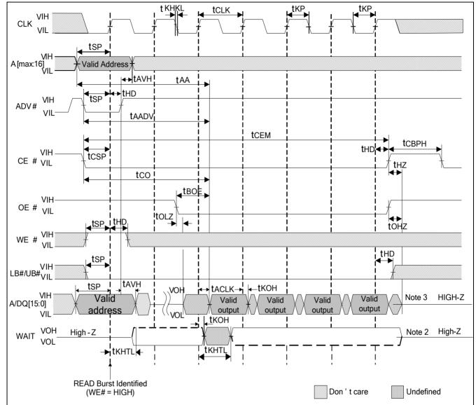
Notes: 1.Non-default BCR settings: fixed latency, latency code 2 (3 clocks), WAIT active LOW, WAIT asserted during delay. 2.WAIT will remain de-asserted even if CE# remains LOW past the end of the defined burst length. 3.A/DQ[15:0] will output undefined data if CE# remains LOW past the end of the defined burst length.
