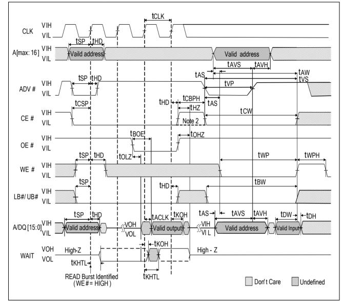
Notes: 1.Non-default BCR settings for burst READ followed by asynchronous WRITE using ADV#: fixed or variable latency, latency code 2 (3 clocks), WAIT active LOW, WAIT asserted during delay.
