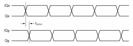
Figure 1c. Output-to-Output Skew
