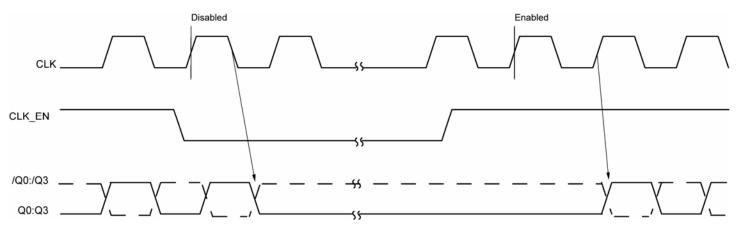
Figure 1a. CLK\_EN Timing Diagram
