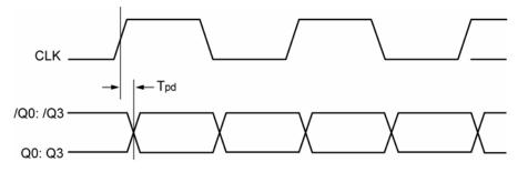
Figure 1b. Propagation Delay
