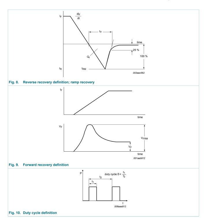
The current ratings for the typical waveforms are calculated according to the equations:  $I_{F(AV)} = I_M \times \delta$  with  $I_M$  defined as peak current,  $I_{RMS} = I_{F(AV)}$  at DC, and  $I_{RMS} = I_M \times \sqrt{\delta}$  with  $I_{RMS}$  defined as RMS current.
